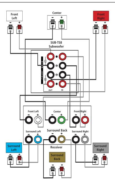
Move the Master Power Switch (marked Power) to the "•" (On) position. The SUB-TS8 subwoofer will automatically turn itself on or go into Standby mode, depending on whether or not a signal is being sent to it by your receiver or surround processor, and provided that the Music-Sense On/Off Switch (3) is moved down so that it is in the AUTO position.
